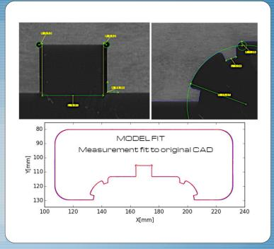
2D Caliper is a two dimensional industrial measurement tool enabling high precision and fast measurements on geometries where it is not possible by conventional digital calipers. D2 provides measurement of complex geometries down to 10um resolution and transfers all measurements directly to CAD format. In matter of minutes, complex part geometry is transferred to digital CAD format and can be compared to original CAD design.
